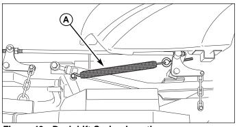
Figure 43. Deck Lift Spring Location
